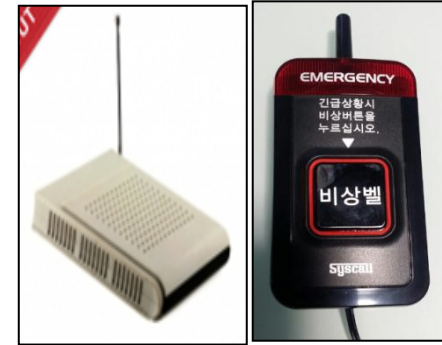
REPEATER – TO BOOST THE SIGNAL
